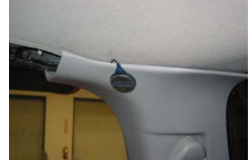
Mount Speaker at top of Driver Side Rear Molding
