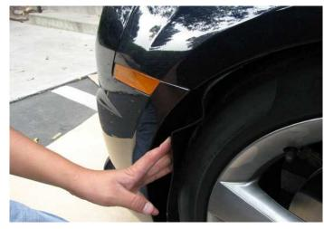
3. Slide off the front fascia but you will to un-plug the wires for the lights. See photo below.
