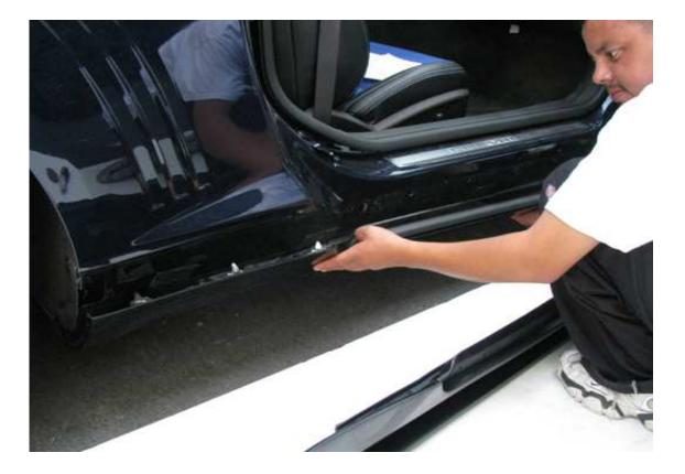
**3.** Next is to get the parts ready to install, You need to sand the tape edge good and then clean with the 3M promoter provided. Below is a photo of the tape lines on the side skirts.
