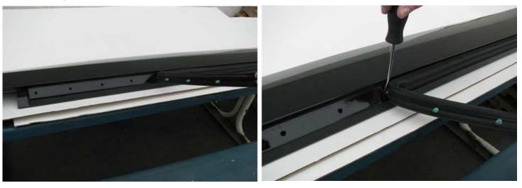
**8.** Next you need to open the door and get ready to install the door seal on to the Street Scene Side Skirt. You will see all of the holes in line. Drill out with a 3/16 drill bit, then you can install the door seal. See photo below.
