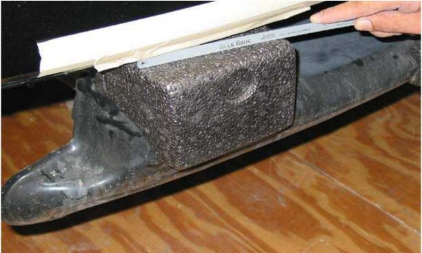
**3.** Install the SS valance by sliding it into position. Re-install the metal retainers to secure the valance. Install the fasteners securing the valance to the inner fenders.
