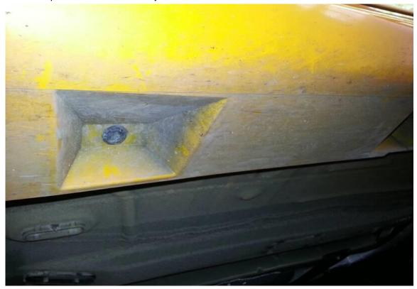
2. Line up the Street Scene Side skirts with the holes and reinstall the Push-Pins into the whole. Repeat the same process on the other side.
