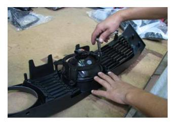
6. Now re-install your new grille shell and install the wires back on the lights. You will need one extension for for the passenger side to reach the plug end. Gently push back into place.
