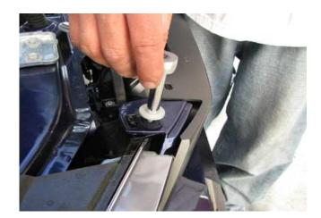
**8.** Replace the air shroud. You will need to slide it under the grille shell then put all of the push in fasteners back into place.
