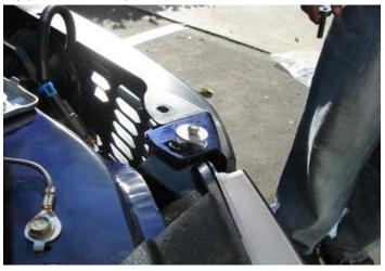
7. Replace the two bolts at each end of shell.
