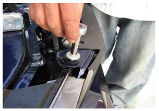
4. Gently pull the factory grille shell away from vehicle and remove the wires to the lights.
