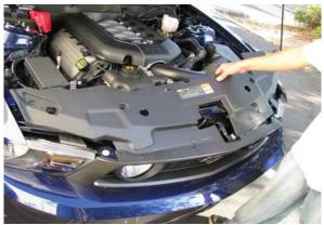
**3.** Release the tabs on the inside of grille shell. There are 6 across the bottom and two on each side. Also remove the two 8 MM bolts at each end of shell. Use a flat blade screwdriver to help to release the tabs.
