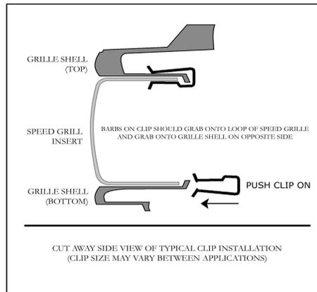
3. Use four clips on each of the side grilles. Use two on the top side and two on the bottom side. The center Speed Grille will require eight clips four on the top side and four on the bottom side. Install clips at each end and center the two others between.
