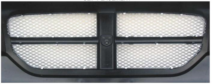
**11.** Install the front fascia in reverse order of removal. Make sure that the top corners of fascia slide into the "T" pins on fenders. Allign fascia to fenders before tightening bolts. Use the six push in fasteners supplied in place of the plastic fasteners that were cut in step four to remove. NOTE: you will not install the two square drive plastic fasteners that were screwed into the styrofoam.
