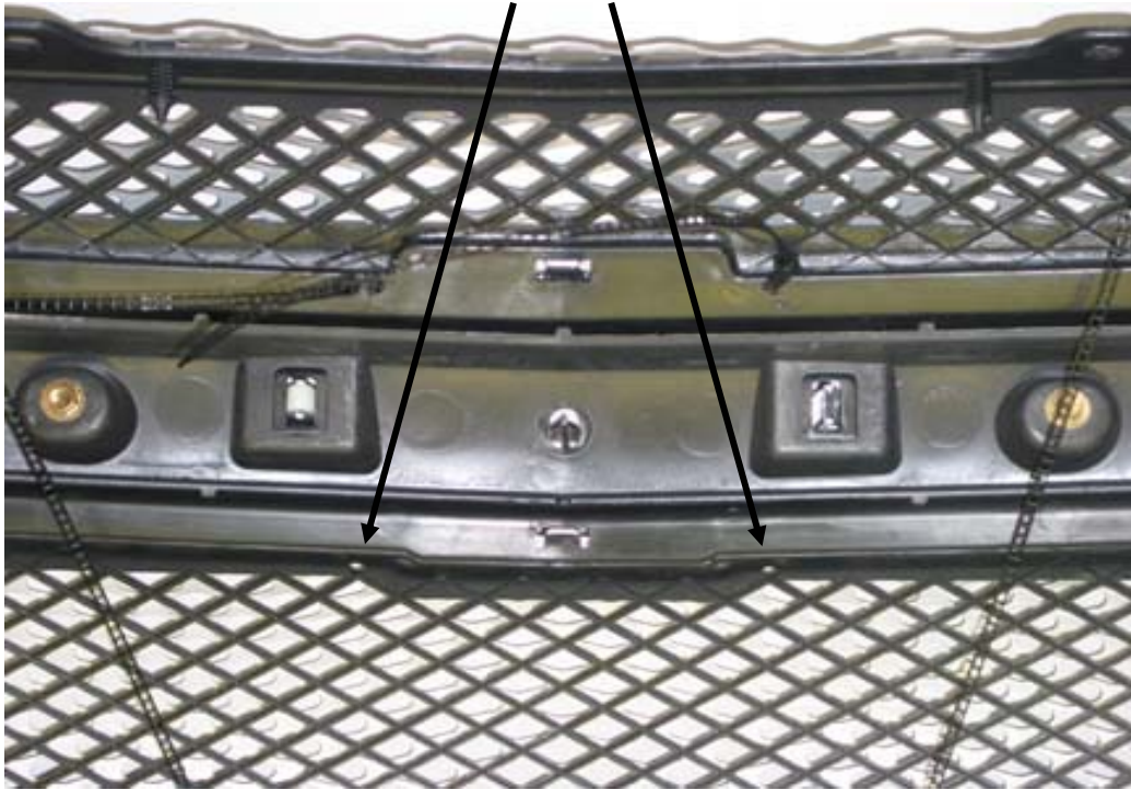
PHOTO 4 Drill Two 3/16" Holes For The Ladders Ties
