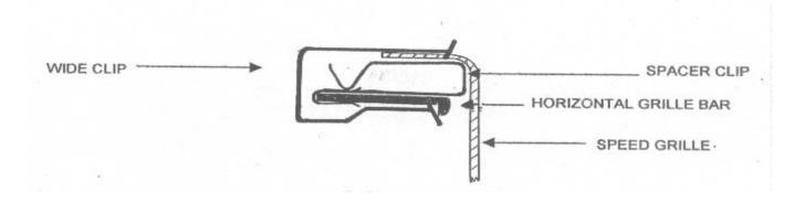
Push grille all the way in. Using the narrow attaching clip, attach the lower side of the "Speed Grille" at the center to the right and left of the "Bow Tie" and at each end one centered between.
