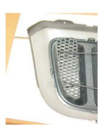
**4.** Install grille shell back on vehicle. NOTE: If the metal mounting clips did not come out when removing the grille, remove them and install on grille shell before installing grille on vehicle.
