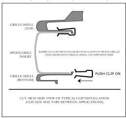
**3.** Install the right and left side Speed Grilles in the same manner, keeping the short side up. Both are identical. Clip to the bumper in the same manner as the center.
