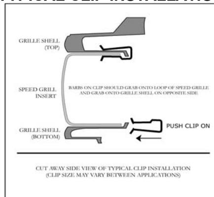
7. Install grille shell back into vehicle by gently pushing at fastening points.
