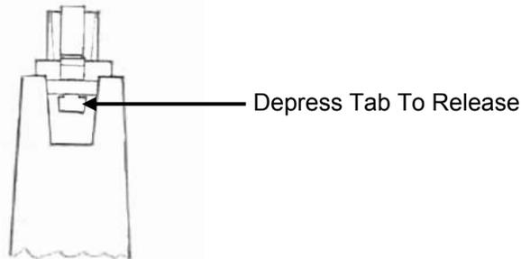
5. Set the grille on a covered bench or table. Remove the Toyota logo by depressing the tab on the top center of logo on backside.
