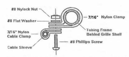
To assemble, first snap the clamps over the cable & tubing. Squeeze the clamps together to insert the #8 screw. Route cable, then tighten.
