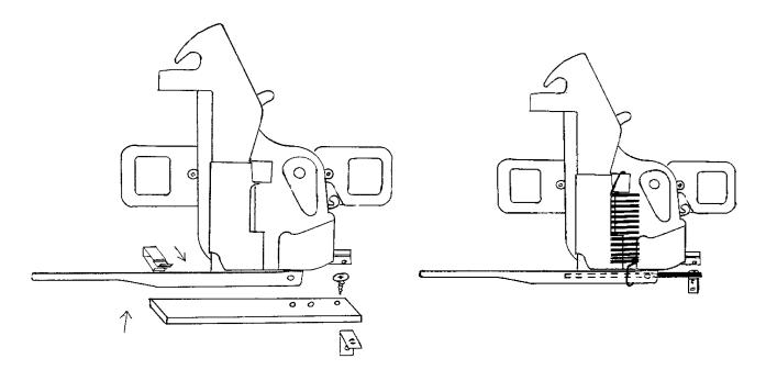
3. Attach the cable clamps to the release cable at each end. Refer to illustration " C " for detail assemble. Attach the cable assemble to the hood release latch assemble with the # 8 phillips head screw, washer and nut.
