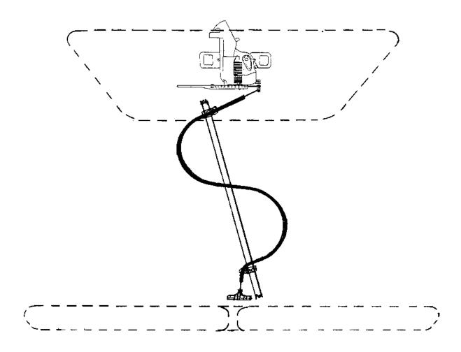
**5.** Attach hood release latch, check for proper operation **BEFORE** installing the Speed Grille.
