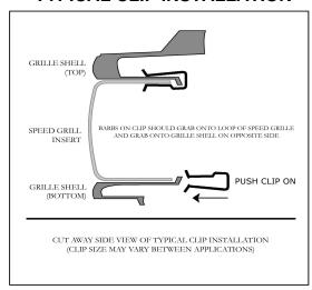
3. Install Grille Sheel back onto vehicle.
