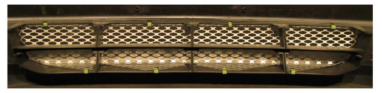
2. Fasten the top of the Speed Grille to the valance lip using the four short installation clips provided. Fasten the bottom side using the longer clips. Clip the bottom at the long extented parts of the Speed Grille. The drawing below will illustrate installing the clips.
