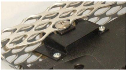
**10.** If you would like to install the GMC emblem cut or grind off the mounting tabs on back side. Apply the two sided tape provided as show in photo below.
