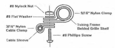
To assemble, first snap the clamps over the cable & tubing. Squeeze the clamps together to insert the #8 screw. Route cable, then tighten.
