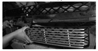
2. Picture shows where brackets should be located.
