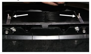
3. Check new grille for firmness and loose hardware prior to driving.
