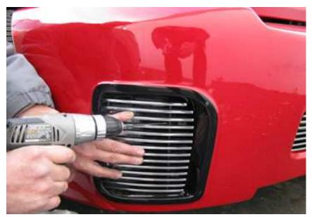
4. Install a phillips head screw into the bumper cover with the retainer nut placed on the back side.
