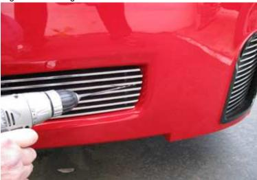
2. Install a phillips head screw into the bumper cover with the retainer nut placed on the back side.
