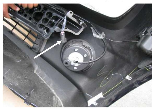
**4.** Now unplug the lights and place the front fascia on a soft cover bench. Hold the Street Scene Splitter in place to see where it will be installed. You will need to clean with the 3M Promoter where the two sided tape will be used. Both the Splitter and the bottom of fascia will need to be cleaned.
