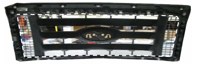
**3.** Use a cut off wheel with disk and cut the inside of the grille shell. Make sure you take your time to do this. Be careful not to scratch the grille shell. After you cut out center sand to a smooth finish.
