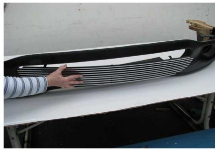
2. Now from the back side center the grille insert where you woulkd like it mounted. Mark the holes and use the hardware provided to mount the insert. You should have the black screws and the tinnerman nuts.
