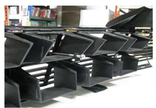
2. From the back side put the L stop bracket on the four bolts and the the nyloc nut. Snug all nuts then make sure the insert strait and tighten all nuts.
