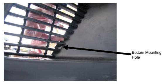
**5.** When using the screw and tinnerman nut screw thru mounting hole and into the side of the urethane then on the other side find the screw and put the tinnerman nut on there and tighten.
