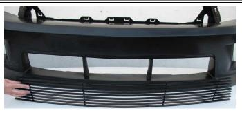
2. From the back side you need to use the hardware provided use the hook bolt and stop bracket and nyloc nut.
