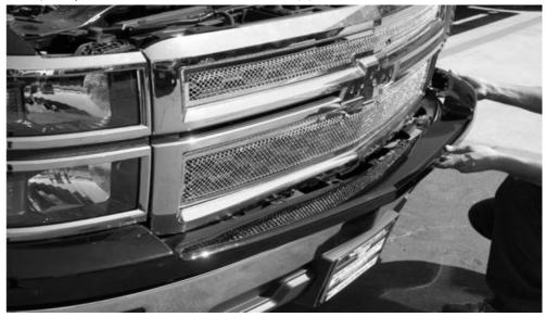
**5.** From underneath of front bumper, use a pry tool to unclip the 4 clips directly underneath the grille shell.
