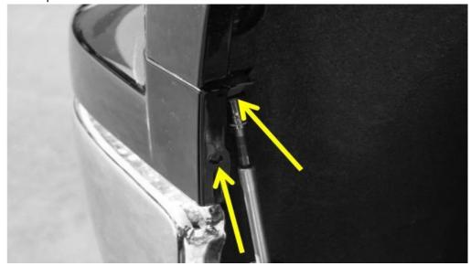
**4.** Use of a plastic pry tool is to push down on clips while simultaneously pulling back on the bumper piece and remove completely from front of vehilce. SEE STEP (5)
