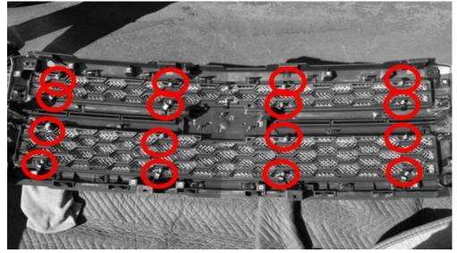
7. Place the "C" bracket as shown and use the lock nut to fasten the grill. Make sure it is secure and DO NOT over tighten. (Repeat Step 5 and 6 for bottom grille)
