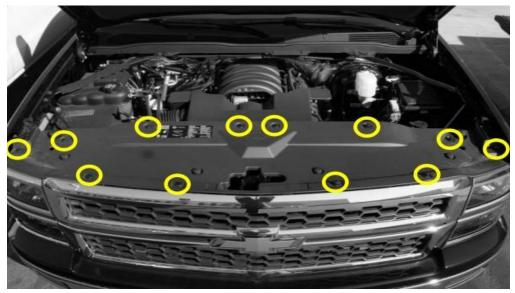
2. With a 10MM socket, remove the 4 bolts from the top of the grille.
