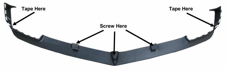
6. With the help of another person place your splitter into postiion where the two sided tape is first. Then where the 3 bosses are you will use the screws provided. Install two in the center boss and one in each of the other two bosses. Use the #10 self tapping screw and on the other side use the tinnerman nut to tighten.
