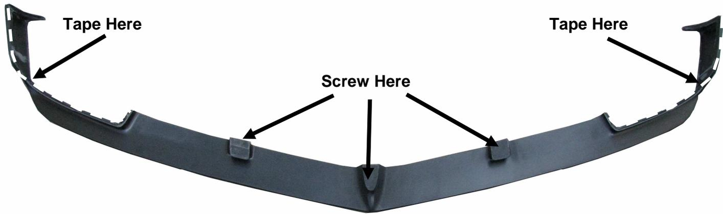
6. With the help of another person place your splitter into position where the two sided tape is first. Then where the 3 bosses are you will use the screws provided. Install two in the center boss and one in each of the other two bosses. Use the #10 self tapping screw and on the other side use the tinnerman nut to tighten.
