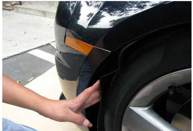
3. Slide off the front fascia but you will have to un-plug the wires for the lights. See photo below.
