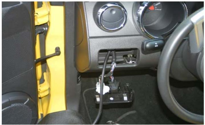
Route the harness wire thru the hole vacated by headlamp switch. See photo 14. Unplug head lamp switch and remove from vehicle.
