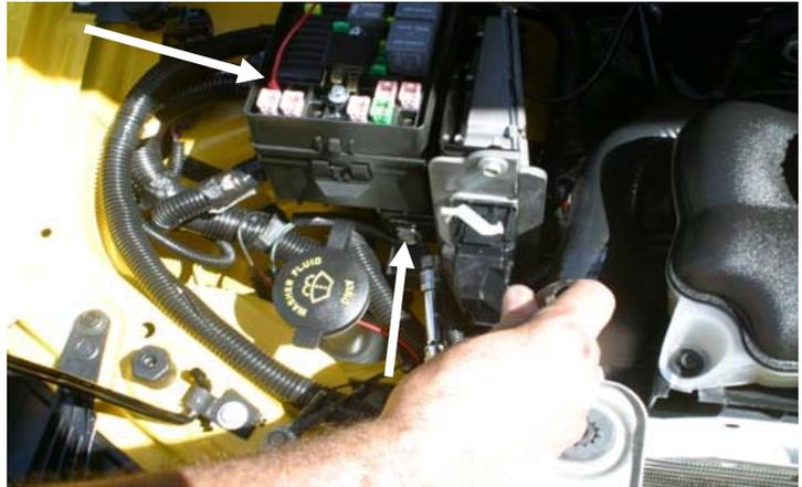
connect the relay to the bolt shown in photo # 5. Make sure to relay plug connection is facing down. If you like you may drill out the hole in relay to 1/4" inch.
