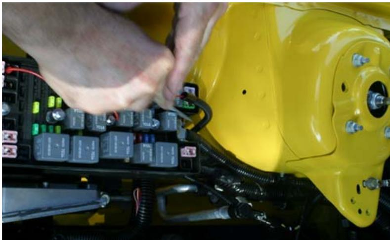
8. Route the harness under the radiator brace ( see photo 8 ) and across the front of vehicle. Make sure the fog lamps plugs are routed to front of vehicle. See photo 9.
