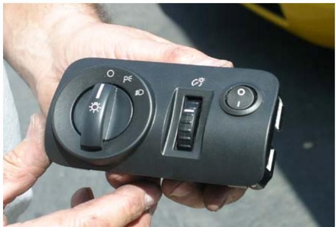
14. Plug the OEM wire harness into head lamp switch. Plug the Street Scene wire harness into the switch install in step 13. Unwrap the black tape on the wires going to the head lamp switch. Locate the RED WITH WHITE STRIPE wire from switch. Connect the RED wire from wire loom to this wire using the Quick Splice connector provided. **DO NOT CUT WIRE** See photo 17.
