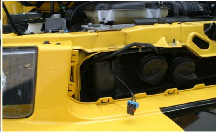
9. Connect the ground wire ( black wire with ring connector ) to the OEM ground bolt on core support. See photo 10
