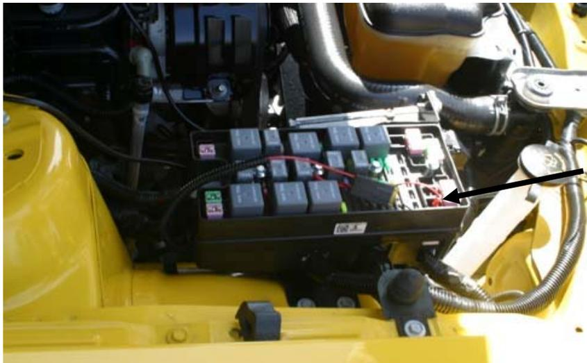
7. File a small slot as shown in photo 7 to run wire into fuse box so that the cover will close See Photo 7.
