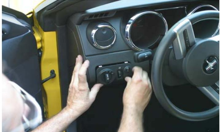
Snap the light switch back into dash. See photo 18. Use the cable ties provided and secure the wire harness under the dash. Be sure to keep harness clear of E brake.
