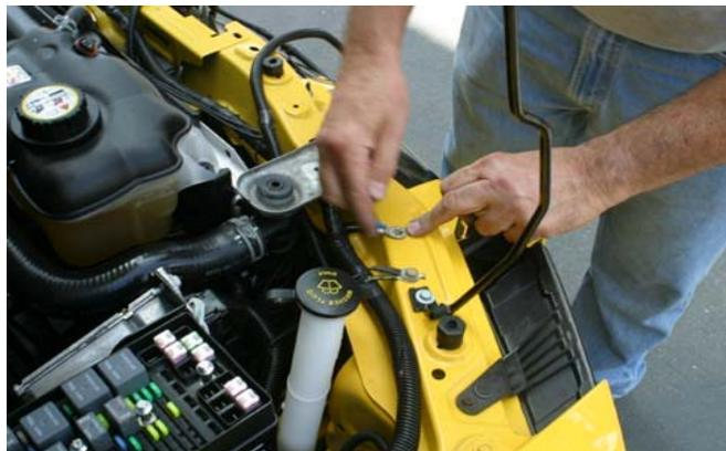
10. Route the remaining harness along the driver's side fender as shown in photo 11, fastening to the hood release cable with the cable ties provided.
