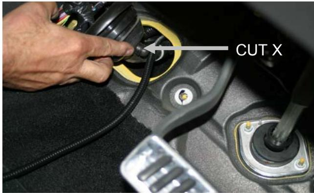
Route the harness down fire wall and through vacated hole. Cut a small X into the rubber boot as indicated by arrow in photo 12. Route the wire harness through this hole and thru boot. Replace rubber boot back into vehicle. Make sure boot is sealed completely in hole.
