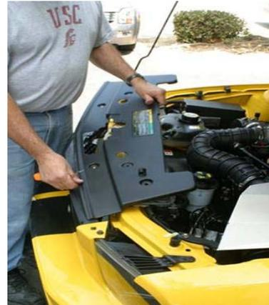
4. Remove the grille from vehicle by pressing the tab on body toward the grille while depressing the tab on the grille shell. Use the flat blade screwdriver to help. See photo 3
